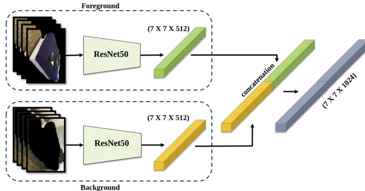
**Fig. 2.** As input, our network takes expanded bounding boxes (see sec. 3.2) which construct a pair of images for masked foreground and masked background (seen on left of image). Each of the pair of images is passed through a ResNet50 where we take an intermediary representation  $7 \times 7 \times 512$  providing spatial information, which is concatenated to provide a joint representation of  $7 \times 7 \times 1024$ .
